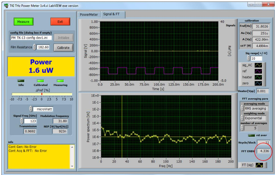
Figure 2.7: The signal and Fourier Transform window, with the Equivalent Noise Bandwidth (ENBW) indicator circled.
