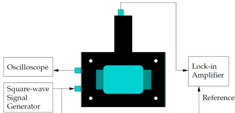
Figure 3.1: Circuit for calibration of the power meter head. An oscilloscope or other peak voltage measuring device attached to the second film connection allows an accurate measurement of the applied voltage,  $V_0$ .
