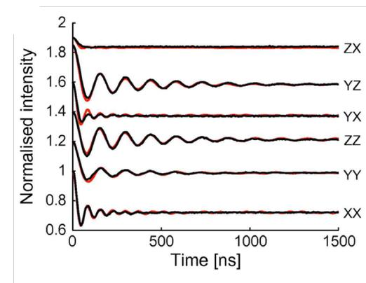
Orientalional PELDOR measurements on a bis-nitroxide model system in o-terphenyl. This highly constrained data set, obtained over 500 MHz bandwidths allows both distance and orientational distributions to be derived.
