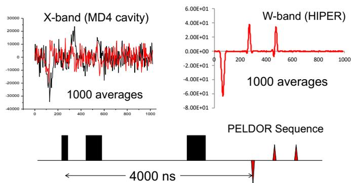
Refocussed spin echo (+ 2 Hahn echos) of 1  $\mu\text{M}$  TEMPO in water glycerol at 50K under conditions typical of a PELDOR measurement. Same fractional number of spins excited.
