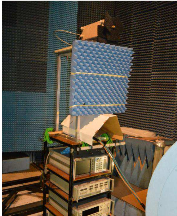
Fig. 2.3 The source antenna on the high platform
