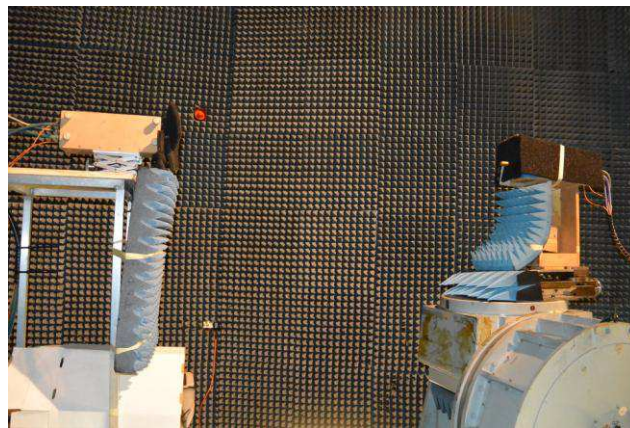
Fig. 2.1 The layout of the far filed test range
