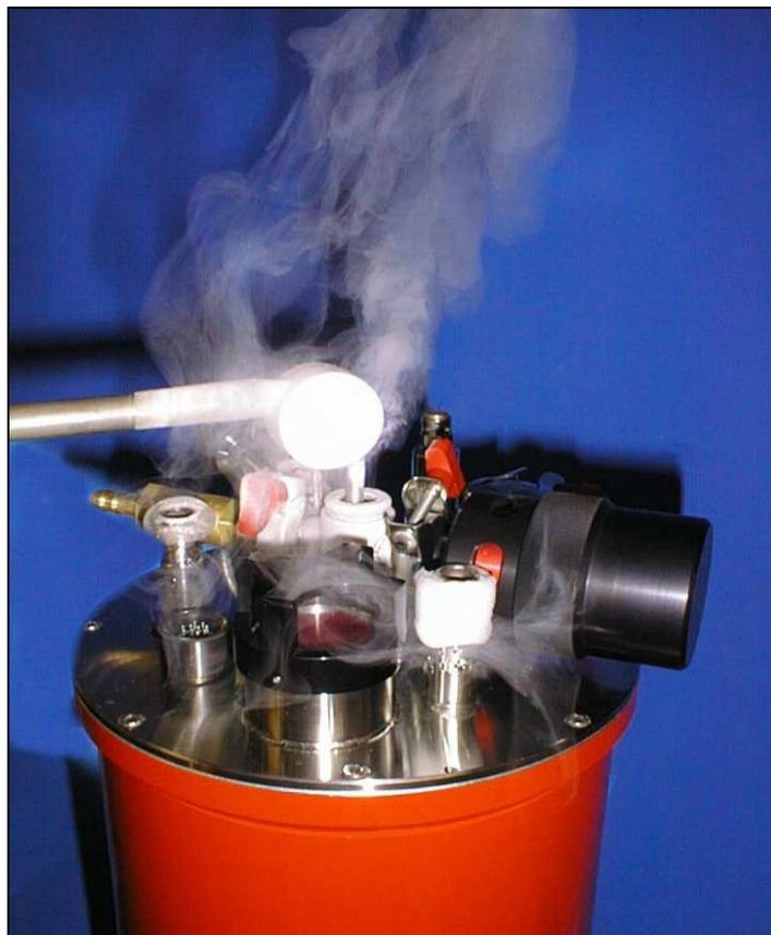
**Photo 4.2.** Helium gas exhaust during fill
