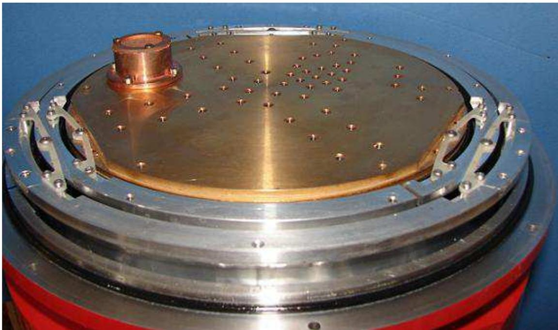
**Photo 1.2.** Cryostat cold plate with the radiation shield extensions removed
