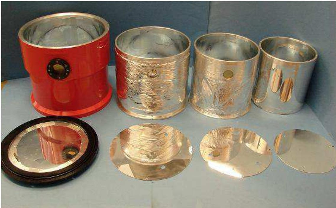
**Photo 1.3.** Cryostat radiation shield extensions and radiation shield base-plates
