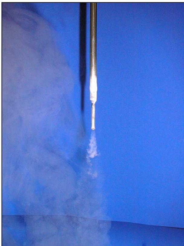
**Photo 4.4.** Liquid helium emerging from a cold tube
