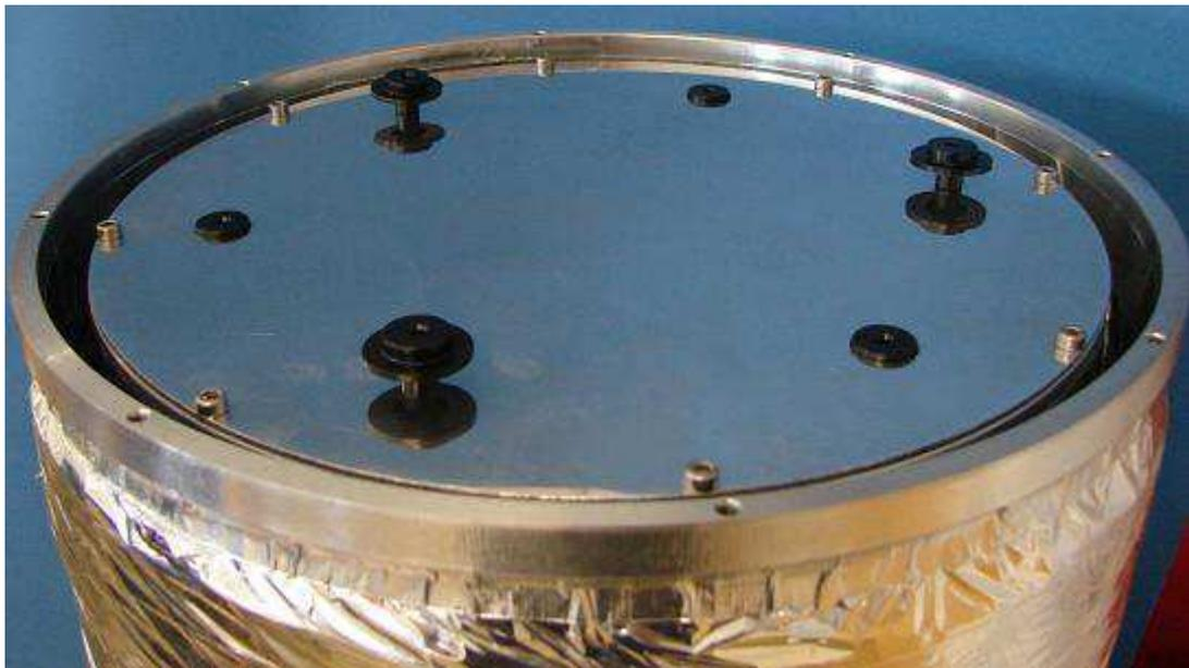
**Photo 1.4.** 77K radiation shield extension mounted on the cryostat along with the 40K gas cooled shield base-plate mounted in position. Note the 3 black nylon spacers used to separate the 4.2K and 40K base-plates, and the 3 black nylon spacers in position for the 77K radiation shield base-plate to be installed.
