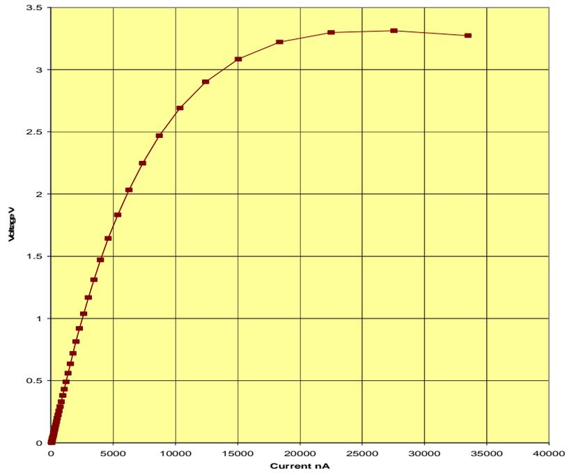
Figure 6.2c Detector VI Characteristic for filter-wheel positions 3, 4 and 5
