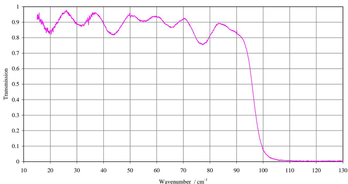
**Fig. C2.** Transmission spectrum for the type QMMF  $100\text{cm}^{-1}$  low pass filter
