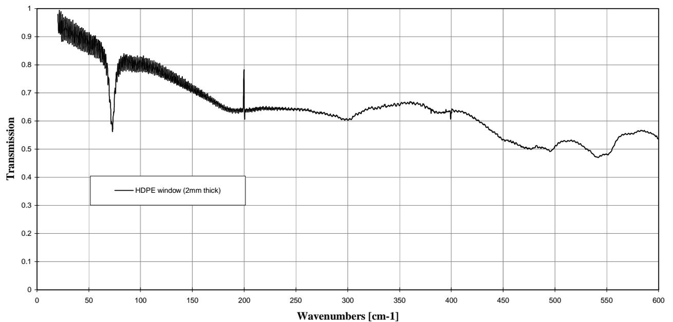
**Fig. C.4.** Measured transmission of a 2mm thick HDPE window from  $20\text{cm}^{-1}$  to  $600\text{cm}^{-1}$ . The polyethylene characteristic absorption increase is clearly seen around  $73\text{cm}^{-1}$
