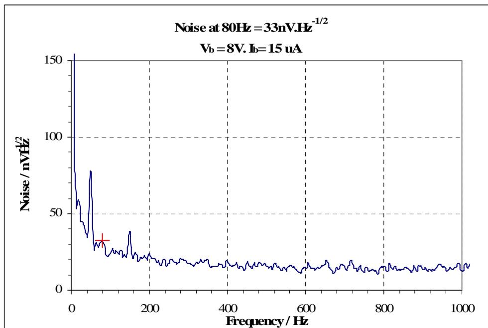
Figure 6.3. System Output Noise Spectrum
