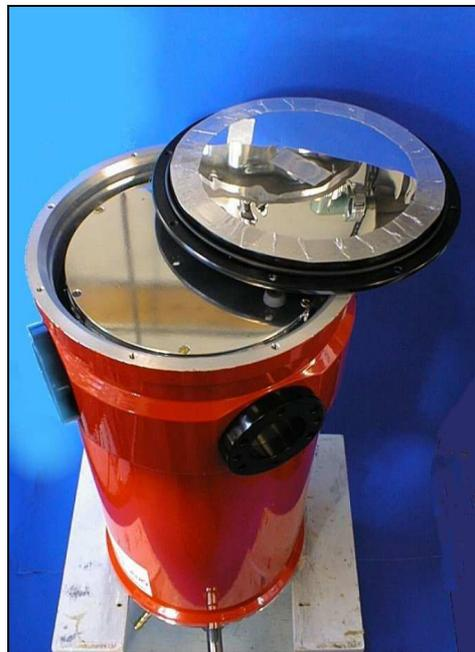
**Photo 1.4.** Liquid nitrogen base-plate in position
