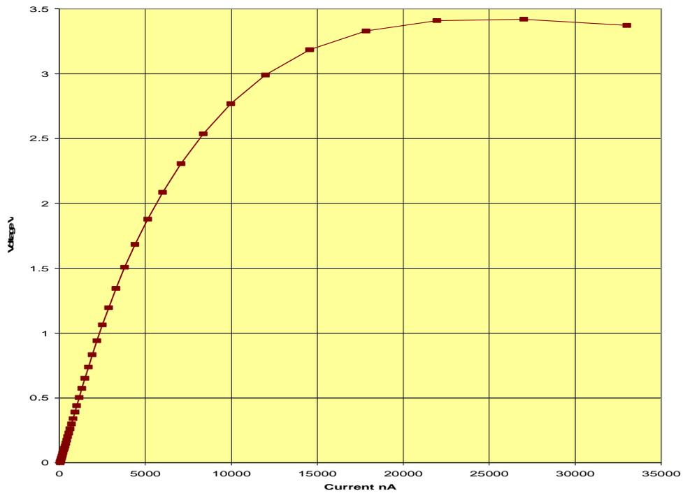
Figure 6.2b Detector VI Characteristic for filter-wheel position 2
