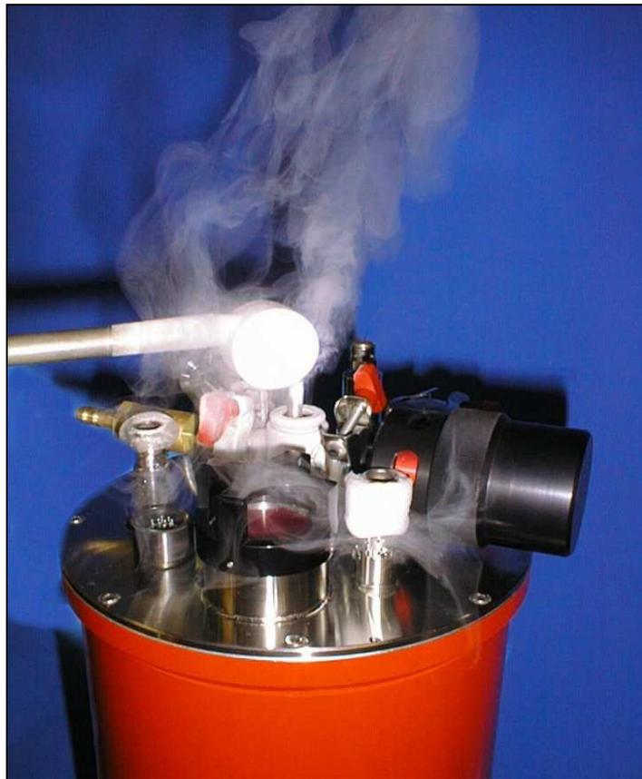
**Photo 4.2.** Helium gas exhaust during fill
