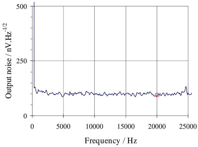
**Fig. 5.1b.** Typical preamplifier input shorted noise spectra
