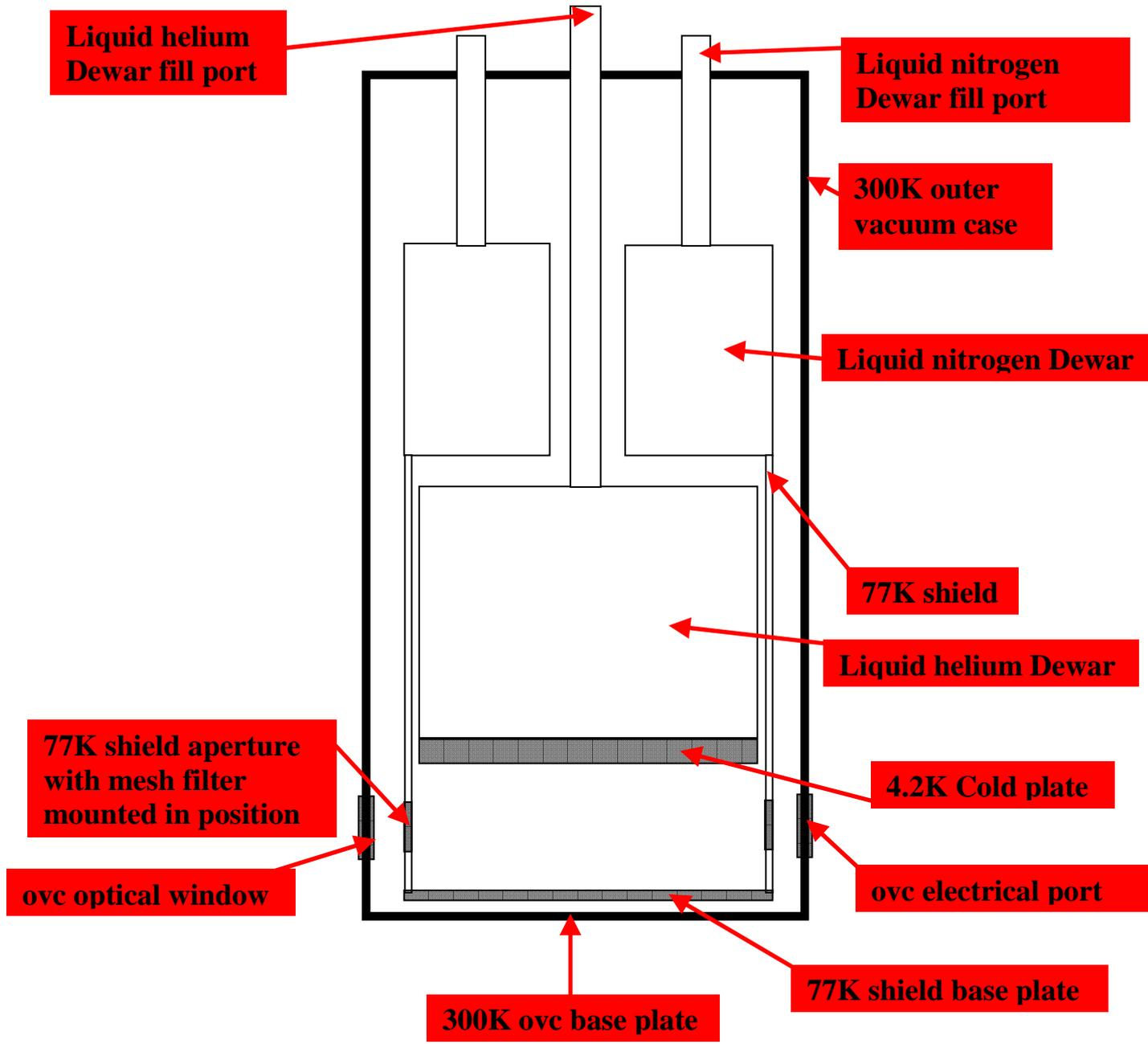
Figure 1.1. Cryostat main features. Not to scale
