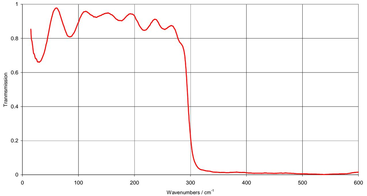
**Fig. C3.** Transmission spectrum for the type QMMF  $300\text{cm}^{-1}$  low pass filter
