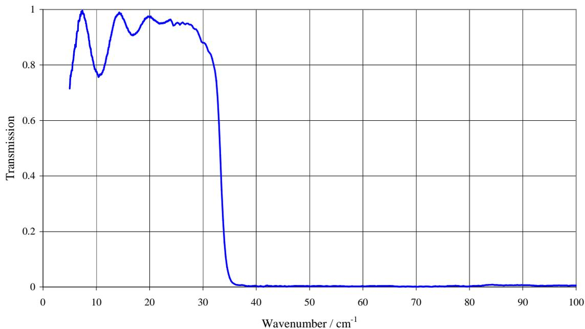
**Fig. C1.** Transmission spectrum for the type QMMF  $33\text{cm}^{-1}$  low pass filter
