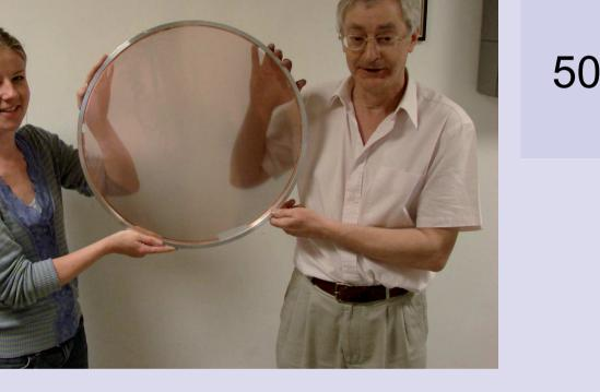
A photolithographic polariser. 500mm in diameter. 10µm pattern period
